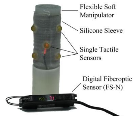
Figure 9: Implemented silicone sensor sleeve with tactile sensors.
