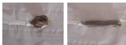
Figure 23: Stiffening membrane in the states of vacuum OFF and vacuum ON.
